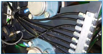
Greasing bearings is extremely important for a long machine life.
