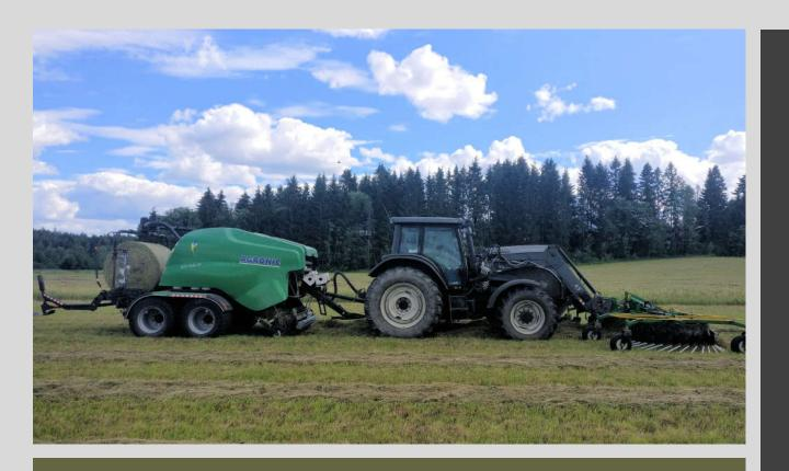
Raking, Baling, & Wrapping: Single Operator. Single Tractor.
