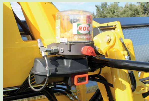
Automatic grease system Optional for all trailed models
