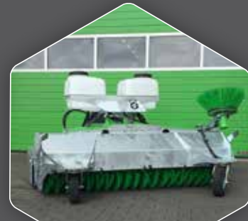
SPRINKLER SYSTEM WITH WATER TANK
